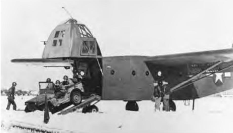
This photo shows how the nose of a glider would swing up to allow for troops and cargo to exit the aircraft quickly after landing.
