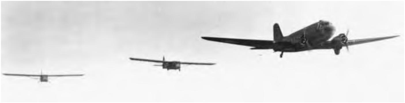
*A C-47 (right) pulls two gliders. Notice that the rear glider has a longer tow line than the one in front.*
