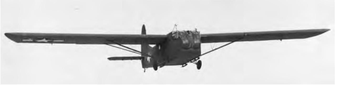
A Waco CG-4A in flight. This nose-on view shows the Plexiglass-enclosed nose that surrounded the pilot and copilot and the struts that braced the wings of the glider. All photos are courtesy of Villaume Industries.
